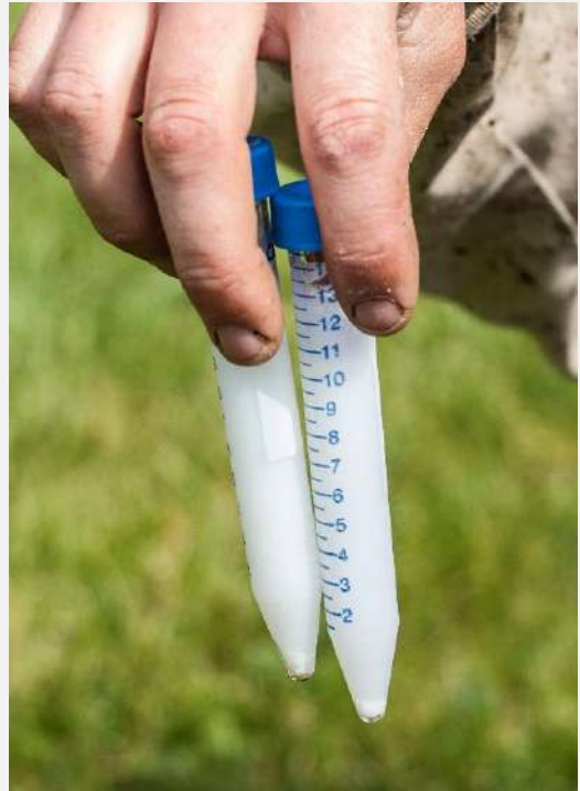
Figure 3: Two tubes filled with dilute milk - one for the test and one as a comparative control. Photo by Sarah Scott.
